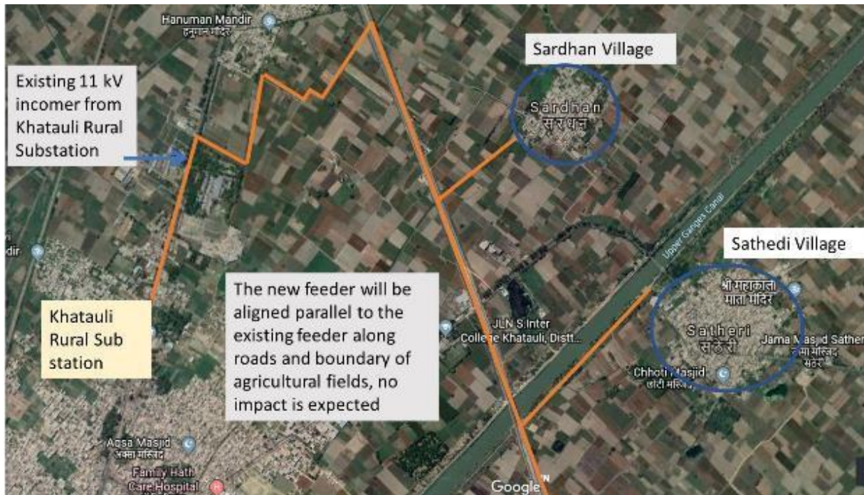
Figure 7: Khatauli Rural Feeder (incomer from 33/11 kV Khatauli Rural substation) in Saharanpur zone in DVVNL
